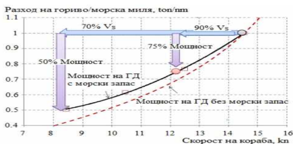
Figure 2. Effect of speed reduction on fuel consumption per mile traveled
