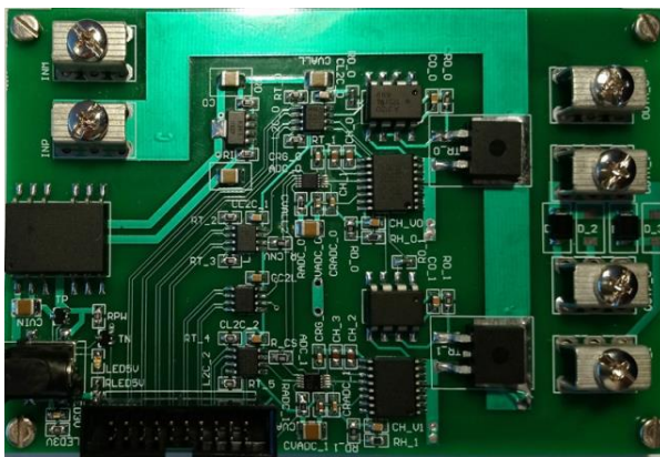
Hardware implementation of the power switching part
