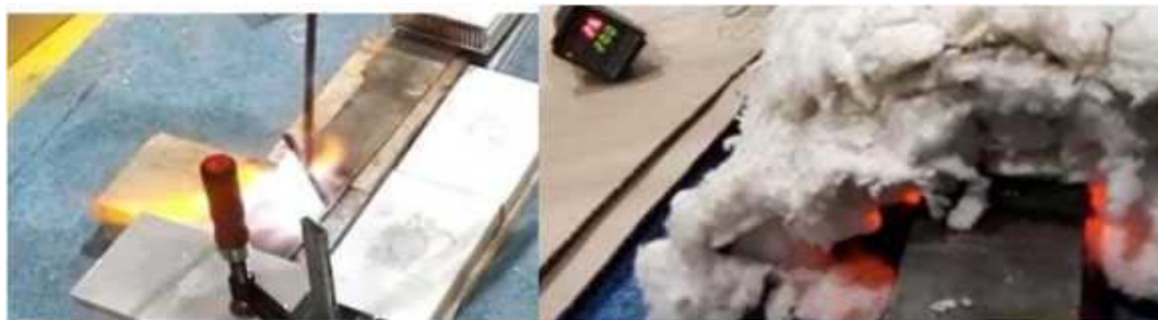
Fig. 54. Flame quenching and subsequent low-temperature quenching retort at 200oC
