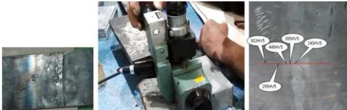
Fig. 53. General view of the welded joint of the GS-50CrV4 (SEW 835) steel rail and the measured Vickers hardnesses HV5.
