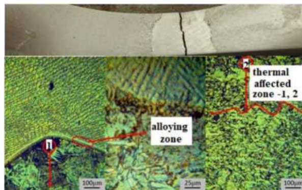
Fig. 16. Microstructures after multicycle fatigue testing
