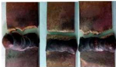
Fig. 38. Tensile strength of welded copper plates
