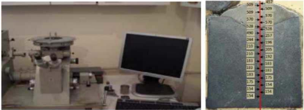
Fig. 31. Metallographic microscope with attachment for measuring Vickers microhardness HV0.05 and the measured hardnesses in transverse section
