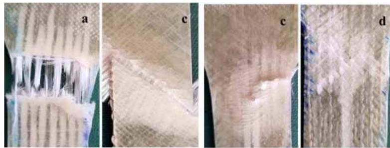
Fig. 11. Macrostructures of the test bodies after testing the strength of bending
