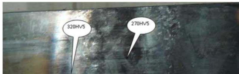
Fig. 55. Results of surface hardness measurements
