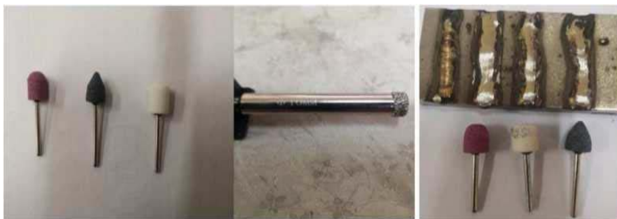
Fig. 58. Used heads for grinding high-speed tool chrome electrocorundum, silicon carbide, white corundum, artificial diamond, welded duplex steel plate.
