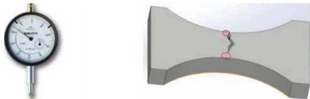
Fig. 48. At least two points are measured with an indicator clock
